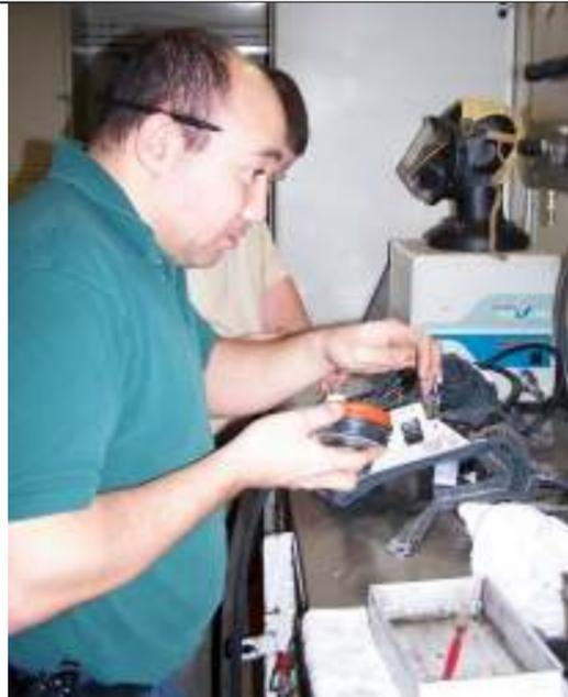
*Technicians from Industrial Protection Supply change out the parts of the airpacks at the Lamoine Fire Station*
